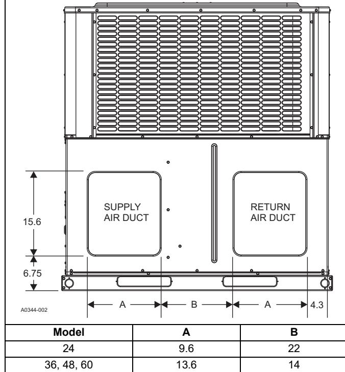
**Unit typical duct applications**
