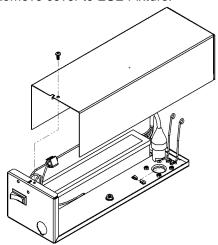
9. Using the fixture base as a template scribe and then create an insertion hole, 2" diameter where you want the emitter to be located.
