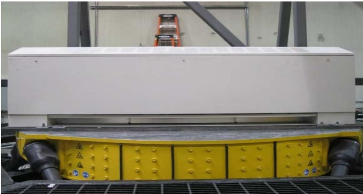
The unit was mounted at the base using four #14 sheet metal screws through the flange at the unit's base. The unit was mounted at the back using the two manufacturer-provided brackets integral to the unit and one 1/2-inch diameter Grade 5 bolt per bracket to attach the unit to the DCL shake table interface frame. The manufacturer-provided brackets at the back of the unit were located at approximately 12 inches from the unit's base.
