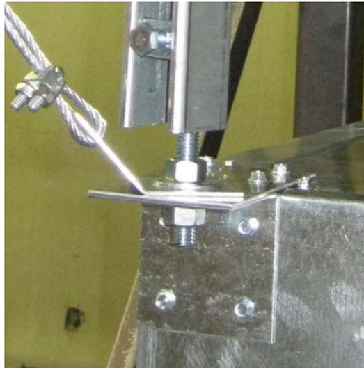
Photograph showing typical mounting for UUT23, UUT26.
