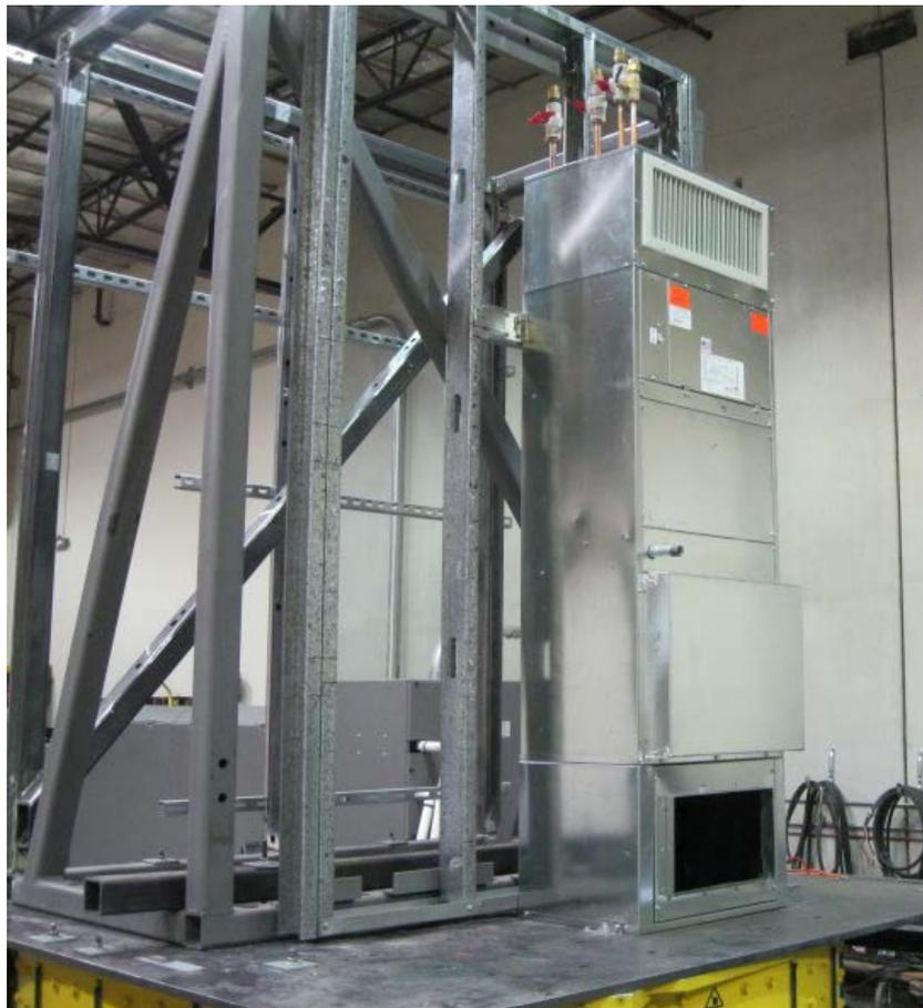
The unit was mounted at the bottom and back using four manufacturer-provided angle clips (one on each bottom-front corner, and one on each side at approximately 55 inches high). Each clip was held in place using five #12, 3/4-inch long sheet metal screws; two screws were attached through the unit, and three through the DCL-provided steel fixture.
