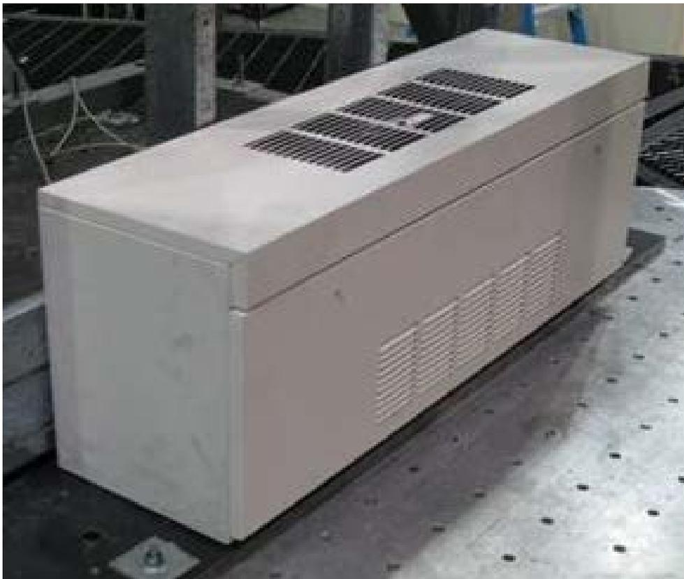
The unit was mounted at the bottom and back using four manufacturer-provided angle clips (one on each front bottom corner and two at the back of the unit at approximately 7 inches high). Each clip was held in place using four #12, 3/4-inch long sheet metal screws; two screws were attached through the unit, and two through the DCL-provided steel fixture.
