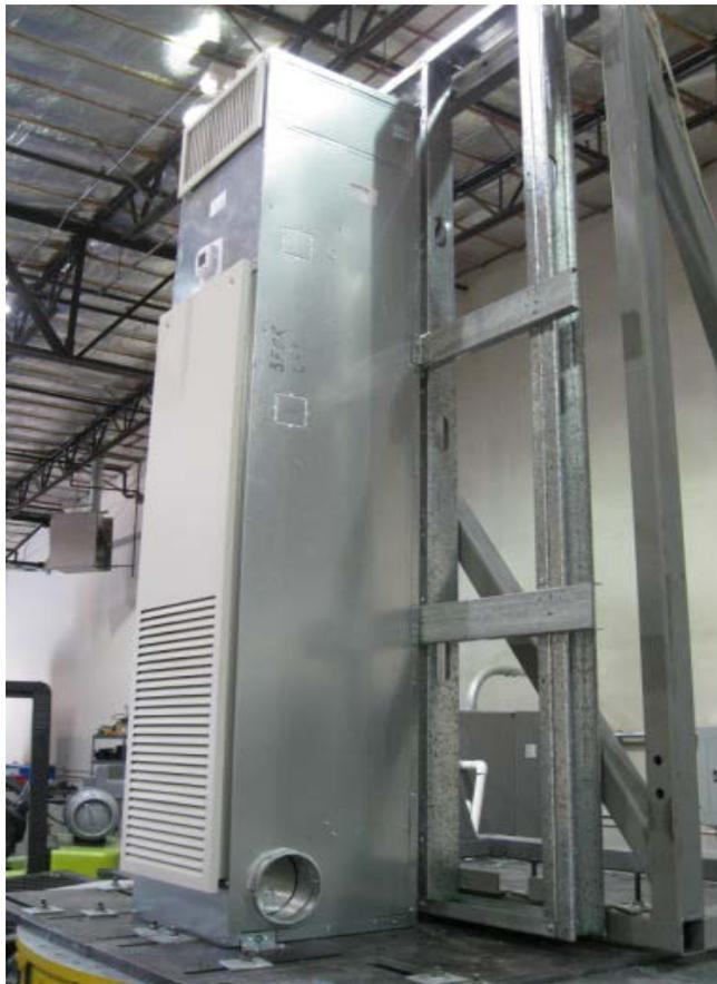
The unit was mounted at the bottom and back using four manufacturer-provided angle clips (two on each front-bottom corner, and one on each side at approximately 58.5 inches high). Each clip was held in place using four #12, 3/4-inch long sheet metal screws; two screws were attached through the unit, and two through the DCL-provided steel fixture.
