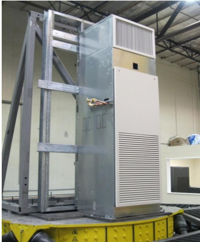
The unit was mounted at the bottom and back using four manufacturer-provided angle clips (two on each front-bottom corner, and one on each side at approximately 58.5 inches high). Each clip was held in place using four #12, 3/4-inch long sheet metal screws; two screws were attached through the unit, and two through the DCL-provided steel fixture.
