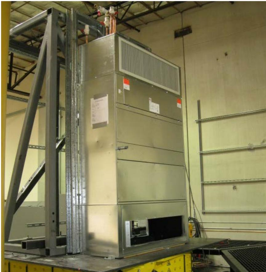
The unit was mounted at the bottom and back using four manufacturer-provided angle clips (two on each front-bottom corner, and one on each side at approximately 58.5 inches high). Each clip was held in place using five #12, 3/4-inch long sheet metal screws; two screws were attached through the unit, and three through the DCL-provided steel fixture.
